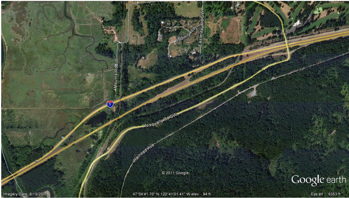
Figure 3. Independent Horizontal Alignment.
